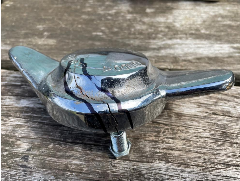
The left hand front wheel spinner, note the split.
